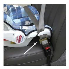
With some cars, you must use a **locking clip** with the lap or shoulder belt. When needed, place the locking clip on both lap and shoulder belts 1/2" to 1" from the latch plate.
